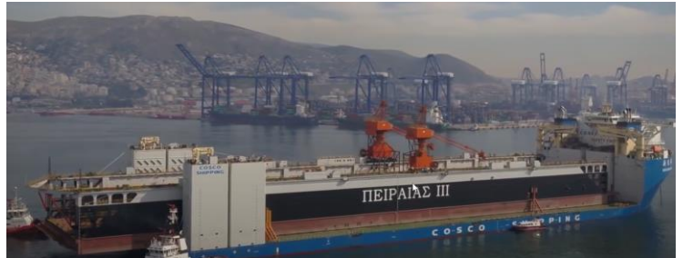
Figure 47: Sea transport of ferries or docks by semi-submersible vessels. [90]
