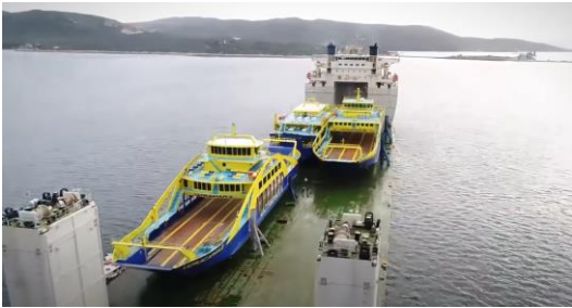
Figure 47: Sea transport of ferries or docks by semi-submersible vessels. [90]
